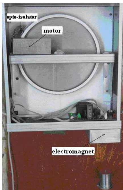
Figure 20. Setup for measuring acceleration (Atwood machine).
